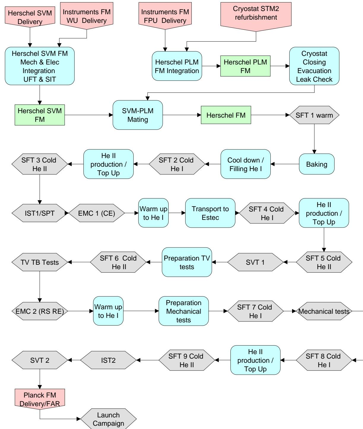
Figure 4-1: Herschel FM test sequence flow chart
