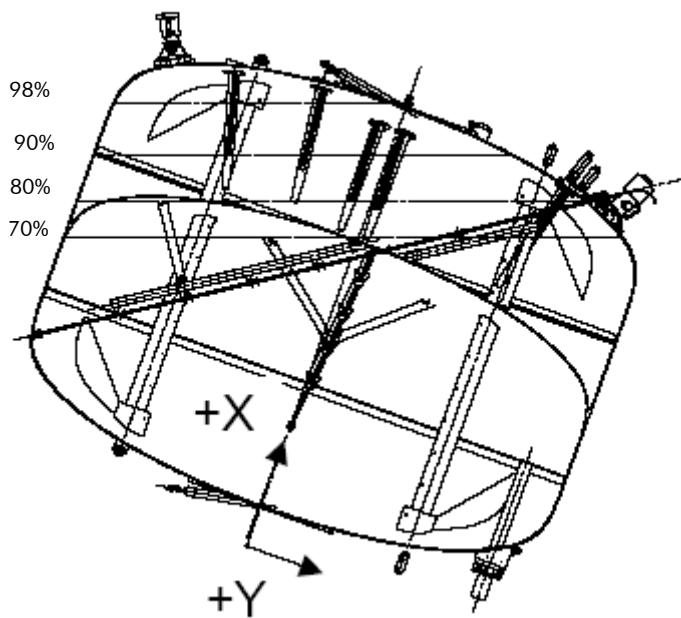
During the IST / Commissioning, the satellite will be tilted, from X vertical, of about +23° around +Z axis (ie +Y goes down) for cooler recycling.
