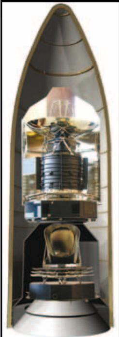
Herschel will be launched on an Ariane 5 along with ESA's Planck observatory, which will study the Cosmic Microwave Background. At launch, the Herschel-Planck combination will measure approximately 11 m high and 4.5 m wide, weighing about 5700 kg. After separating from the upper stage, the two spacecraft will head towards their respective orbits. They will be operated independently.
