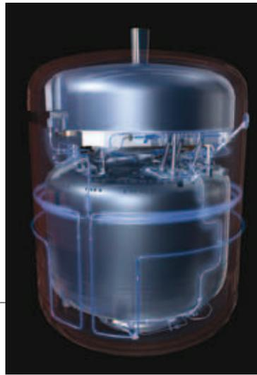
The gas continues into the rings of the shields, cooling them down to 30K ( $-241^{\circ}\text{C}$ ), 50K ( $-221^{\circ}\text{C}$ ) and 60K ( $-211^{\circ}\text{C}$ ), respectively.
