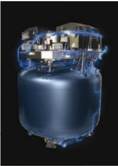
Herschel's superfluid helium tank, where the helium is kept at its boiling temperature (1.65K or  $-271.5^{\circ}\text{C}$ ). The helium cools the focal plane unit of the scientific instruments and the three thermal shields. The liquid boils and produces gas that slowly flows from the tank into pipes around the payload, cooling it to between 1.7K ( $-271.4^{\circ}\text{C}$ ) and 4K ( $-269^{\circ}\text{C}$ ).
