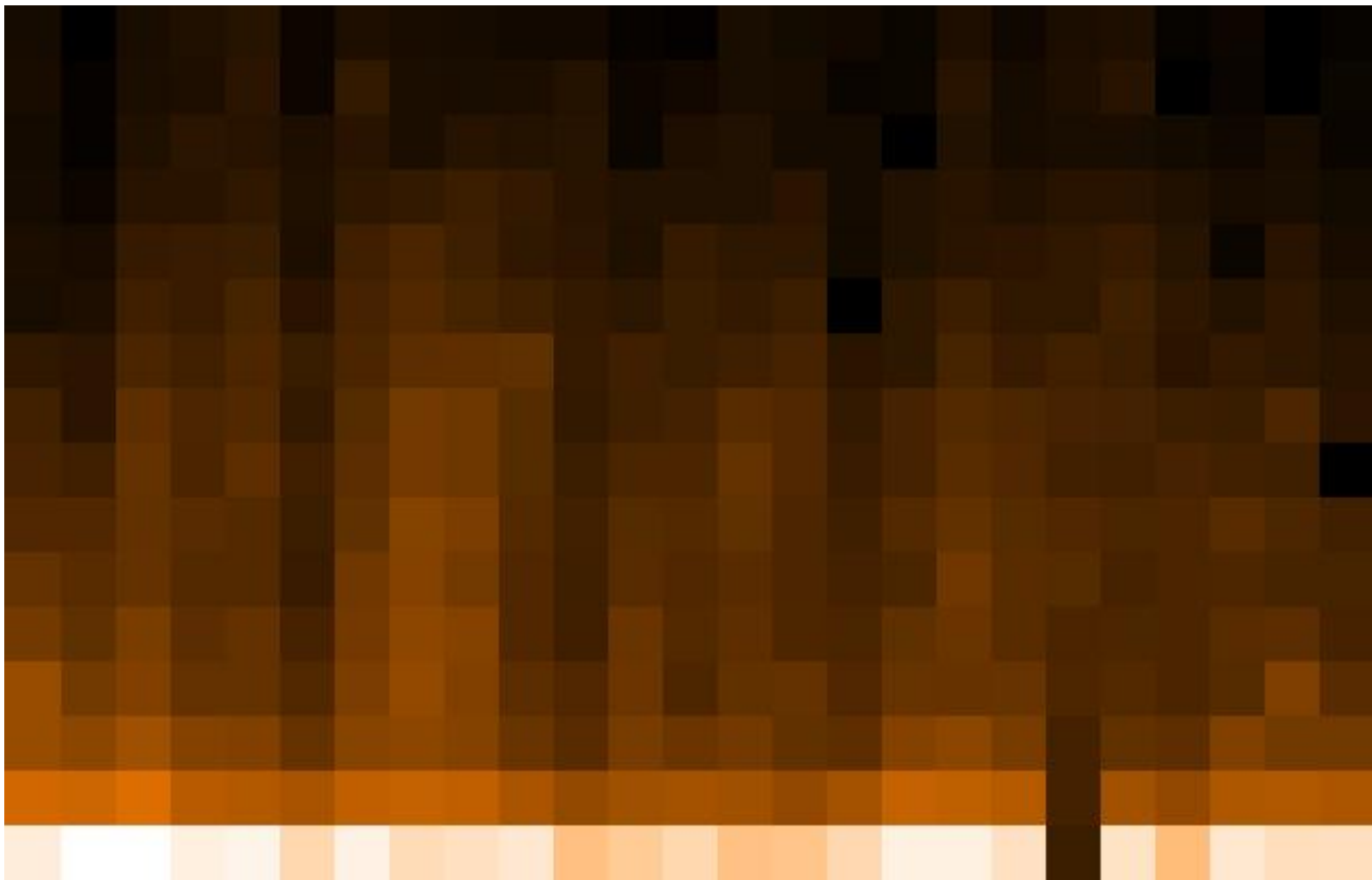
Figure 4: The mean dark current frame for the last exposure in the blue array. The higher dark current in rows 15 and 16 is due to a crosstalk effect with the dummy channel (row 17).
