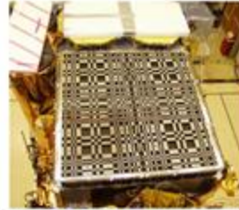
The IBIS coded mask, placed at 3.2m from detector. Built using 16mm thick W blocks, min.size 11.2mm
