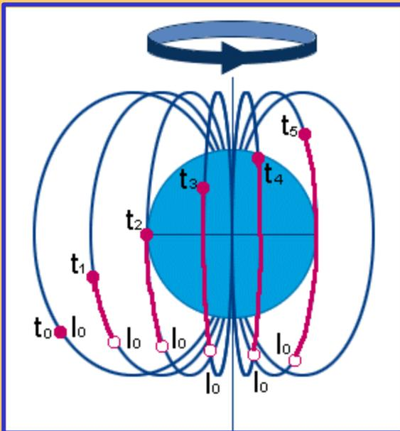
*RESONANCE satellite motion along the selected magnetic flux tube, mapping to the heating station.*
