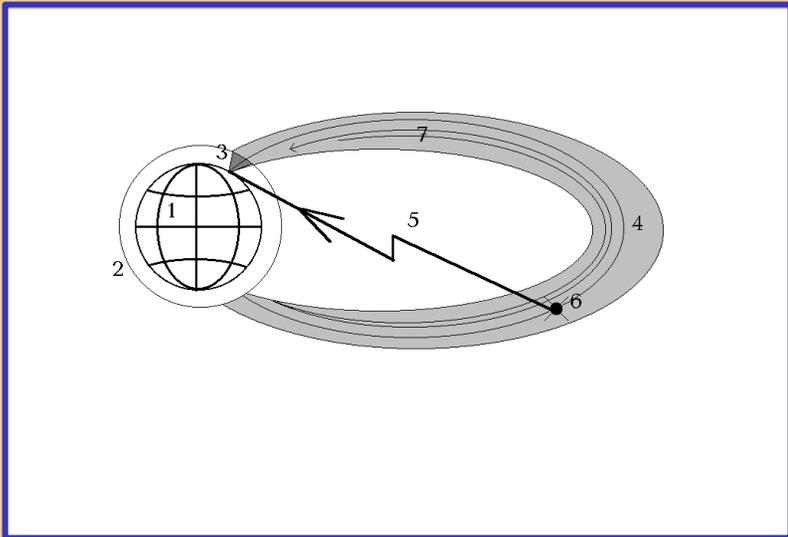
Controlled positive or negative feedback will be added to the natural magnetospheric oscillator by means of real-time communication with the heating station
