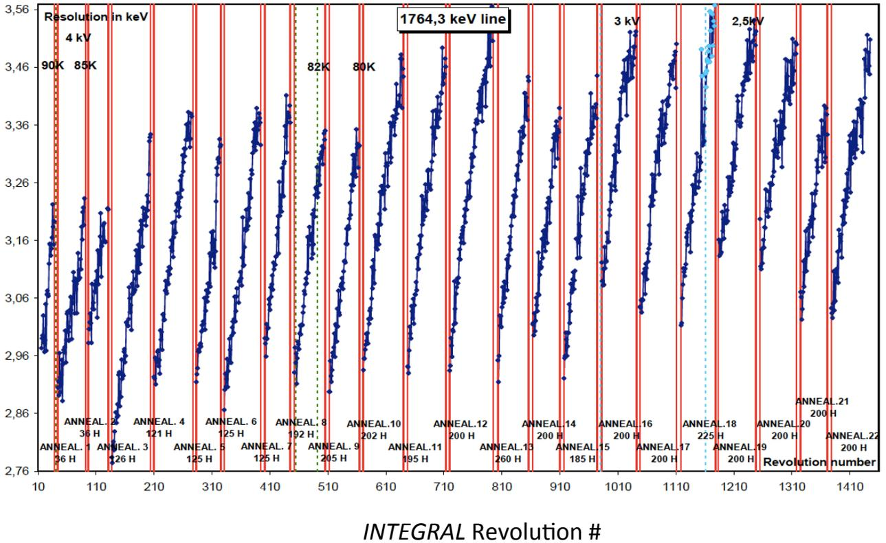
**Figure A6:** Evolution of the SPI energy resolution at 1764.3 keV since end of commissioning phase (orbital revolution #10). Until September 2014, twenty-three annealing cycles (red vertical bars) have been successfully performed consistently recovering the nominal pre-launch energy resolution.
