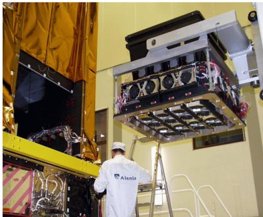
*The IBIS detector unit is being integrated into the spacecraft's payload module at ESTEC, November 2001.*
