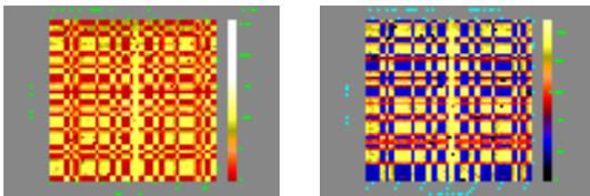
*First shadowgram obtained with the IBIS telescope at ESTEC. Radioactive sources (60 keV, ISGRI [left] and 661 keV, PICSIT [right]) were used to cast shadowgrams of the IBIS coded aperture mask onto the ISGRI and PICSIT detector arrays.*
