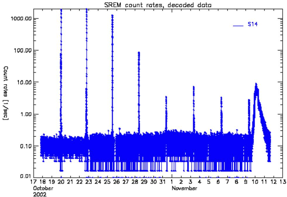
Figure 1: Proton count rates measured by IREM from switch on until mid November. Clearly visible is the reduction in the proton flux by almost 3 orders of magnitude from the initial transfer orbit to the final orbit. The broad feature around November 9th is associated with solar activity. Courtesy: P. Buehler and the IREM team.
