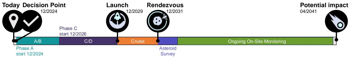
Recommendation: Start, as soon as possible, the initial design phases (phases A/B) of in-space mitigation missions, based on the following concepts, including the risk assessment on each option: kinetic impactor (KI) and ion beam deflection (IBD).
