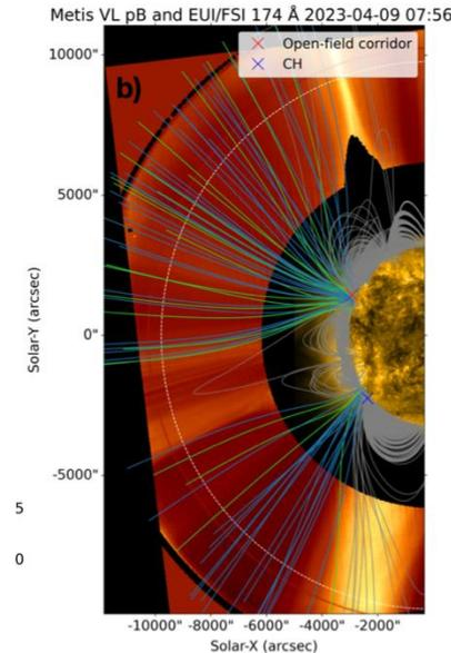
The magnetic field extrapolations derived from the PSI-MAS MHD simulation during Carrington rotation 2269.
