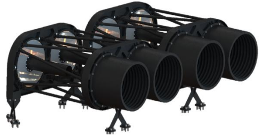
Figure 8: The ARRAKIHS instrument with two iSIM170 binocular telescopes
