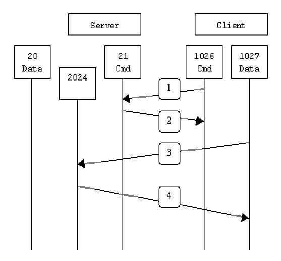
In step 1, the client contacts the server on the command port and issues the PASV command. The server then replies in step 2 with PORT 2024, telling the client which port it is listening to for the data connection. In step 3 the client then initiates the data connection from its data port to the specified server data port. Finally, the server sends back an ACK in step 4 to the client's data port.
