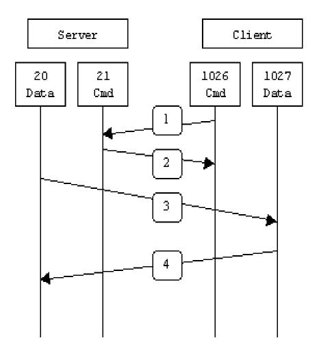
In step 1, the client's command port contacts the server's command port and sends the command PORT 1027. The server then sends an ACK back to the client's command port in step 2. In step 3 the server
